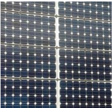
Cellule monocristalline (source CAUE60)
